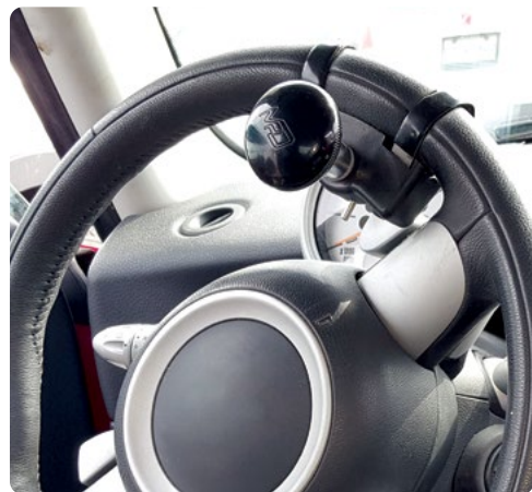
Installing a spinner knob on your car's steering wheel may be required if stipulated during an assessment.
