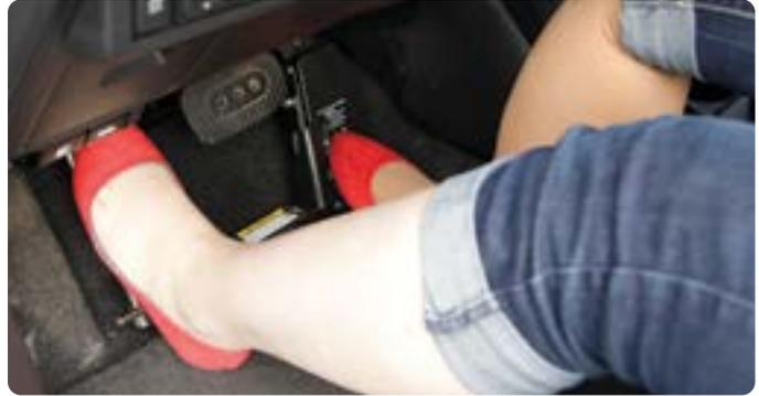
**A pedal extender can be used to help drive.**
